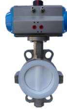
Wafer Split Body Concentric Butterfly Valve Fig.2310 Standard: BS5155/EN593/MSS SP-67/API609 Size:DN50~DN600
